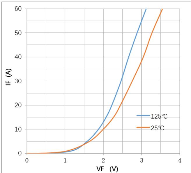
Figure8: typical diode forward characteristic,  $t_p=300\mu\text{s}$
