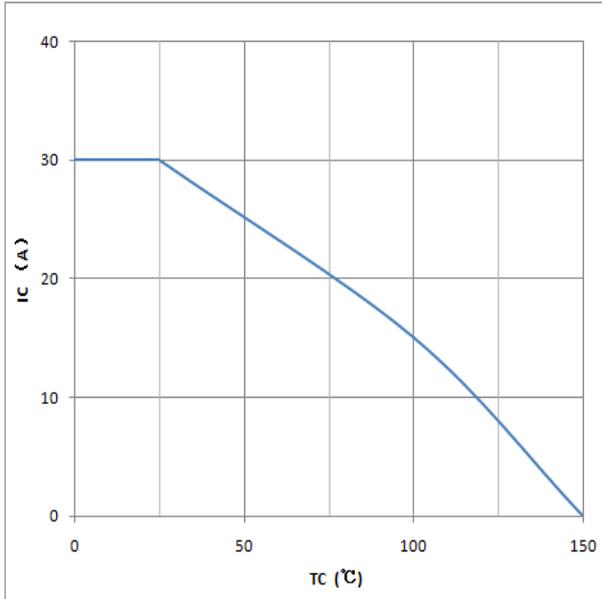
Figure1: maximum DC collector current VS. case temperature
