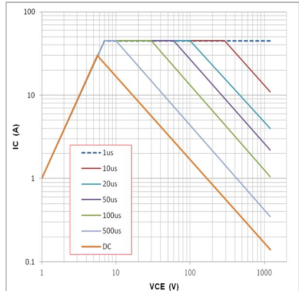
Figure4: forward SOA,  $T_C=25^{\circ}\text{C}$ ,  $T_J \leq 150^{\circ}\text{C}$
