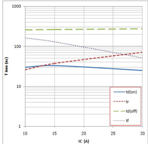
Figure10: typical switching time VS. IC, TC=25°C,
