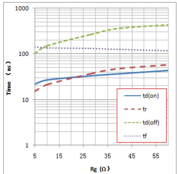
Figure12: typical switching time VS. Rg, TC=25°C,
