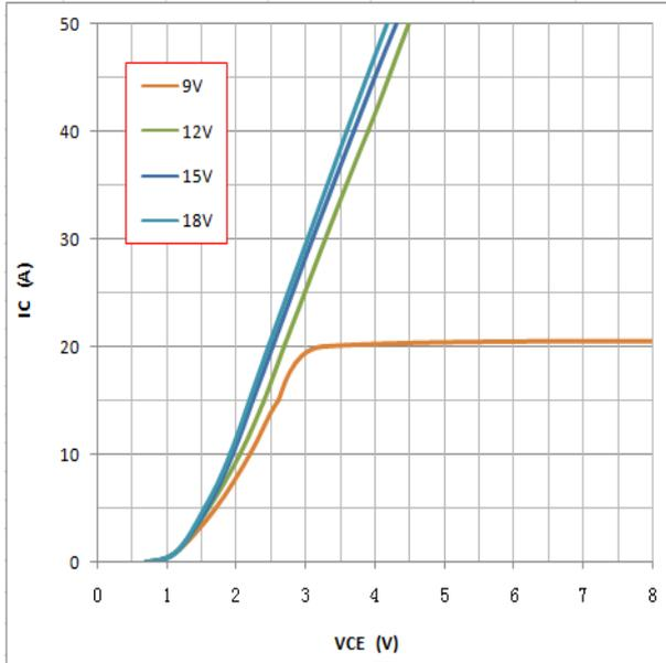
Figure5: typical IGBT output characteristics,
