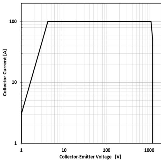
Figure 3. Reverse bias SOA,  $T_j=125^{\circ}\text{C}$ ,  $V_{ge}=15\text{V}$
