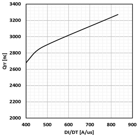
Figure 15. Typical diode Qrr vs di/dt Tc=25°C
