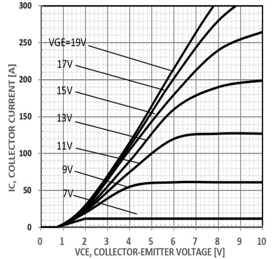
Figure 6. Typical output characteristics
