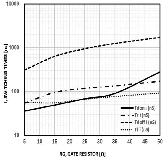
Figure 10. Typical switching time VS. Rg, TC=25°C,
