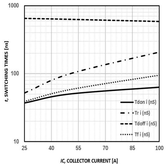
Figure 12. Typical switching time VS. IC,
