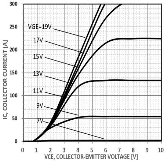
Figure 5. Typical output characteristics
