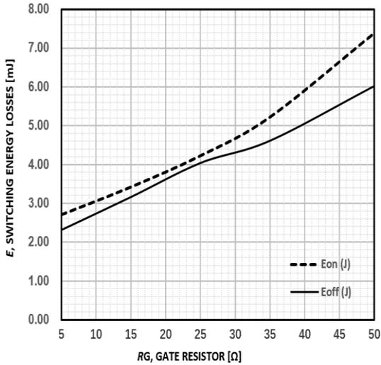
Figure 9. Typical energy loss VS. Rg, TC=25°C,
