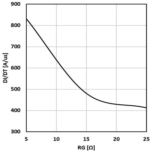
Figure 13. Typical diode di/dt vs rg Tc=25°C
