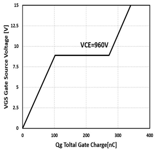
Figure 4. Typical gate charge VS.  $V_{GE}$ ,  $I_C=50\text{A}$
